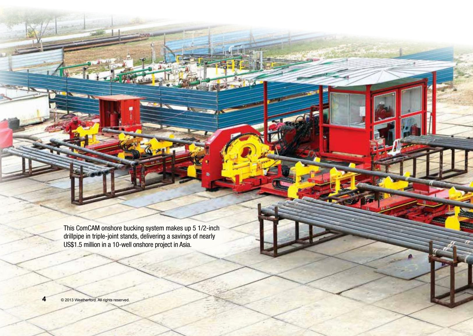
This ComCAM onshore bucking system makes up 5 1/2-inch drillpipe in triple-joint stands, delivering a savings of nearly US\$1.5 million in a 10-well onshore project in Asia.
