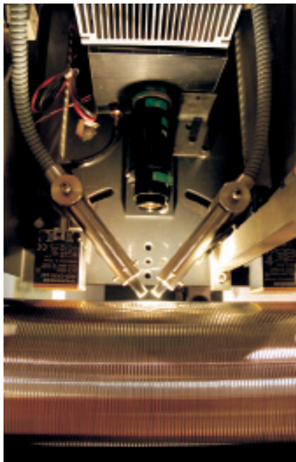
Photometric inspection system measures wire, spacing the full length of each screen to meet client specifications.
