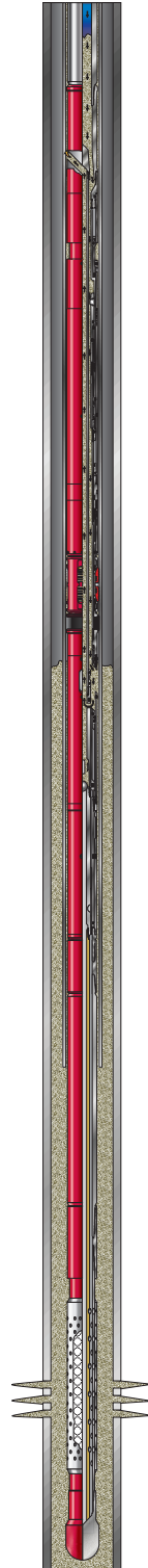
Screenout opens circulating ports and circulates out excess gravel
