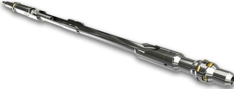
The advanced kickover tool incorporates many unique features, including highly efficient rollers which eliminate contact friction, enabling access to gas-lift mandrels located at higher deviations. Reduced friction also delivers a more precise indication at the surface of the toolstring load transfer, enabling the slickline operator to identify toolstring movement more easily and make improved decisions to reduce the chance of a misrun.
