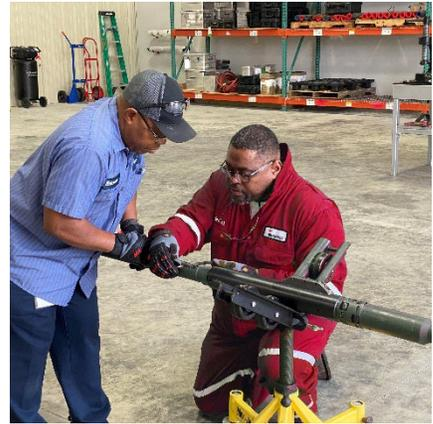
Pinning the engineered arm of the advanced kickover tool avoids misruns during deployment. When activated, the arm engages the gas-lift valves at the correct approach angle and avoids damage to the V-packing seals when setting gas-lift valves.
