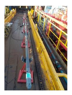
Weatherford ISO-Flex high-expansion retrievable bridge plug provides a robust and reliable well barrier with minimum deployment operational time. The ISO-Flex system is a mechanical barrier with a large, direct-to-the-wellbore equalization area that is ideal for sub-hydrostatic applications. Its multi-conveyance methods allows for deep or shallow deployment, setting, and retrieval using industry-standard conveyance techniques for added speed and simplicity.
