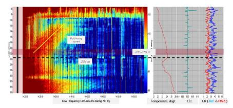
High-resolution, low-frequency DAS detects upward flow movement. This suggests fluid is leaking through the production casing and migrating upward within the annulus. The temperature anomaly at this depth further supports this interpretation
