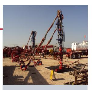
Weatherford used a hybrid water-fracturing technique on 15 wells in the Chicontepec Basin, Mexico, enabling the operator to realize a 20% cumulative production increase over conventional fracturing treatments.
