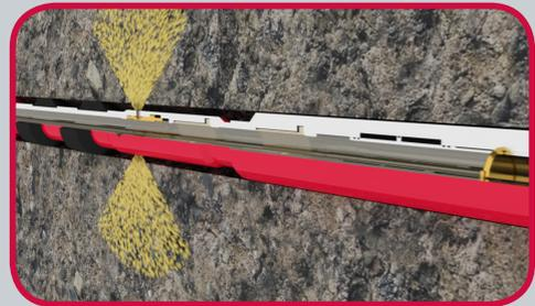
Figure 2: Main Frac through RFID ARID Sleeve
