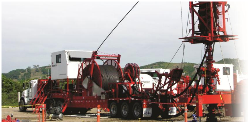
Working in a difficult lateral section, Weatherford provided an efficient alternative to a plug-and-perf completion using only a coiled-tubing unit.
