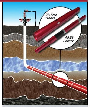
Weatherford's ARES openhole packers and *ZoneSelect* technology isolated 21 individual zones in a 20,111-ft (6130-m) lateral well, decreasing overall costs while increasing production rates.
