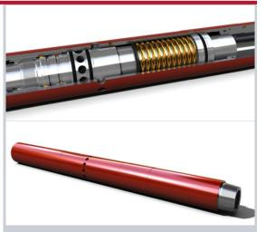
Weatherford ZoneSelect SMART Toe Sleeve allows the casing string to be tested to its full working pressure, with an unlimited hold period and without exceeding the working pressure. Placed at the bottom of the completion string, the SMART toe sleeve actuates and opens after two internal pressure applications. Once the SMART toe sleeve is open, ZoneSelect composite plugs can be pumped downhole for stimulation.
