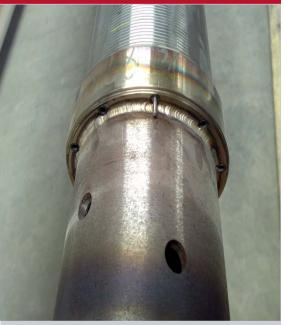
Weatherford's *ZoneSelect* completion system with *ASP GENESIS* packers and *FloReg* ICDs enabled multiple isolations to be performed in a single trip without thru-tubing intervention, reducing water production and enabling a more uniform flow throughout the 14,800-ft (4,511-m) horizontal well.
