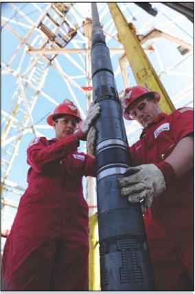
The Weatherford *OptiPkr*, one component of the *Optimum* completion system, is a premium high-performance production packer that offers the robustness of a permanent packer with the flexibility/versatility of a retrievable packer.
