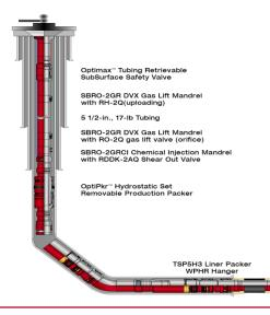
Weatherford's *Optimum* upper-completion system mitigates the elevated risk, and potentially expensive consequences, of performance failure in harsh environments. An integrated array of highly durable upper-completion components, including an interventionless removable production packer, subsurface safety valve, multiple downhole control valves, and flow-control equipment are designed to work in tandem for reliability, efficiency, and life-of-well performance.
