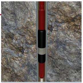
The Weatherford single-set, rotation release, injection production packer greatly enhanced well safety by providing a temporary seal while the surface equipment was changed. This solution for the odd-sized casing in the well enabled full well access while running in the hole.
