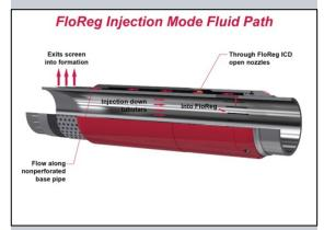
Weatherford's *FloReg* ICD provides uniform inflow distribution in horizontal and deviated wellbores and reduces water or gas production for more efficient reservoir drainage.
