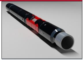
Weatherford's patented openhole *ROKANKOR* system is an innovative design that uses six mechanical slips to grip the formation with limited penetration, minimizing fracture damage in the immediate contact area during the setting event.
