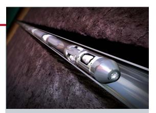
Weatherford's ESS technology is a better option for a narrow window between pore and frac gradients. Traditional openhole gravel packs are susceptible to fracturing the formation whereas ESS technology will not, ensuring a stabilized wellbore and a low-skin completion with excellent sand control. Expansion is achieved from the surface with proprietary compliant expansion tools.
