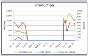
The graph shows that after the installation of *MazeFlo* technology, the oil production increased significantly and gas production remained similar. Water production and sand management were eliminated.
