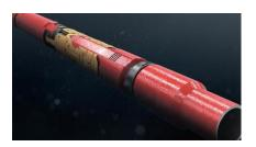
The ROk-ANKOR slip system is a unique tool that keeps the completion string from moving during stimulation or production operations. It also prevents open-hole packers from sliding up or down the wellbore, eliminating wear and thus increasing their reliability and overall life span.
