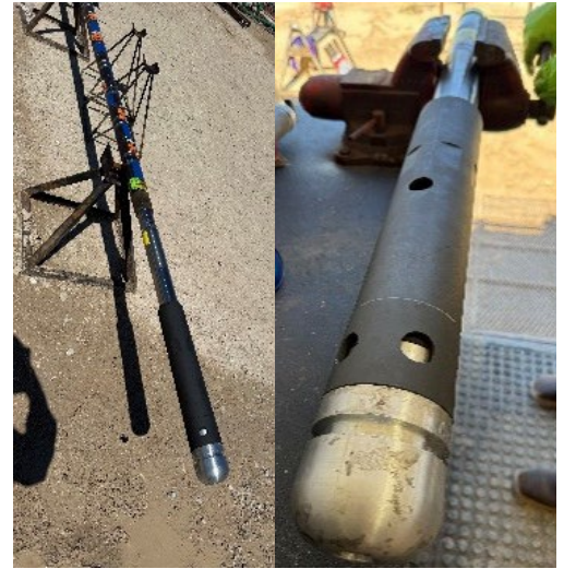
Zone seal plug made up to standard pump-down BHA prior to deployment.
