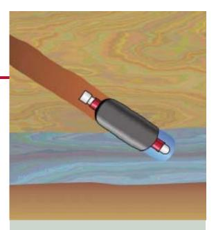
Weatherford's ACP annulus casing packer can be used to plug and abandon a section of a wellbore completely after drilling at the end of a horizontal section.
