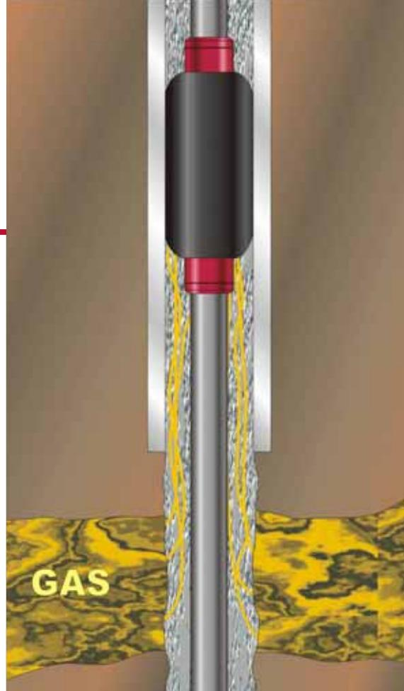
Weatherford's ACP annulus casing packer provides a proven, reliable solution for isolating zones and mitigating blowout risks.
