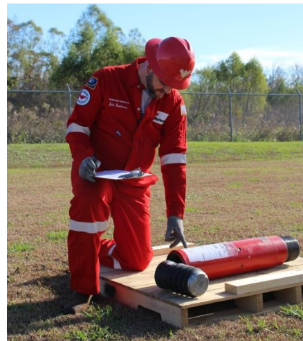
The Weatherford Eliminator GT series stage tool (Model 756) has hydraulically opened ports that enabled both stimulation and cementing through an 80° deviation.
