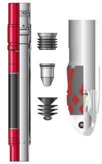
The Weatherford POST (left and middle) features an inflatable packer element that creates a barrier to enable second-stage cement to go to the surface even in total losses. The DiamondBack reamer shoe (right) features a diamond-shaped tungsten-carbide cutting structure that provides a 360° cutting radius.
