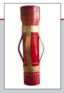
Weatherford's Model 541R bow-spring centralizer subs passed through a 17.77-in. wellhead clearance and centralized a 17-in. liner in 20-in. open hole, enabling ConocoPhillips Norway to achieve a successful cement job for long-term zonal isolation.
