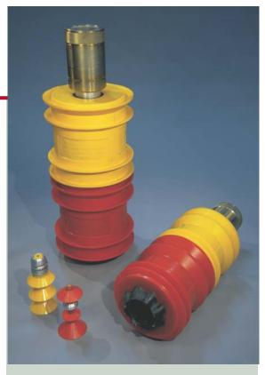
Weatherford's *Sub-Surface Release* plug system is primarily polyurethane and contains very little aluminum. These properties greatly reduce the amount of time needed to drill up equipment, in some cases reducing it to less than two hours.
