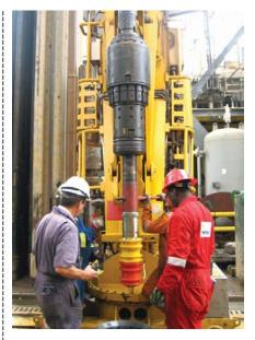
Weatherford SSR plug systems are designed for use with Weatherford autofill float equipment and SurgeMaster diverter tools, which are run to reduce surge pressures and increase running speeds.
