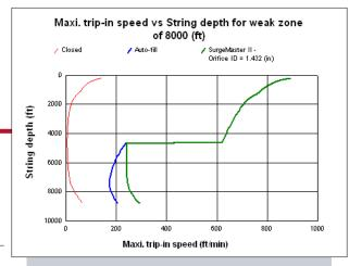
SurgeMaster<sup>™</sup> II multiple-opening diverter tool reduced surge pressure, increased running speeds (as shown in this chart), and decreased potential safety hazards by directing mud into the annulus above the casing or liner.
