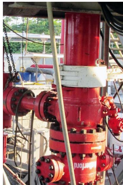
The SafeShield® Model 7100 rotating control device (RCD) enabled use of managed pressure drilling techniques to drill through the depleted hole section.
