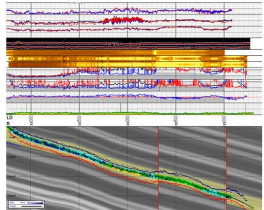
Using a sourceless azimuthal sonic and resistivity BHA, Weatherford successfully delivered two 6-in. lateral wells despite a high degree of geologic uncertainty.
