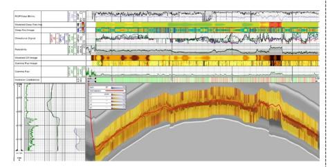
The GuideWave CLEAR service delivers the highest confidence with less uncertainty for precision steering decisions in clastic and carbonate reservoirs by providing a multi-boundary inversion with a deterministic approach that calculates the thickness and resistivity of the formations in a radius exceeding 40 ft (12.1 m) around.
