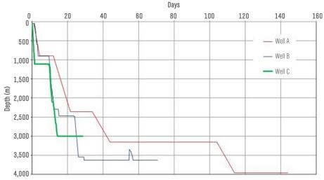
The above graph illustrates the delivery of three wells in the same field. Weatherford Integrated Services delivered Well C (green) with just two casing sizes in approximately 25 days. By comparison, competitors delivered Well A (red) and Well B (blue) with four and three casing sizes in approximately 145 and 72 days, respectively.
