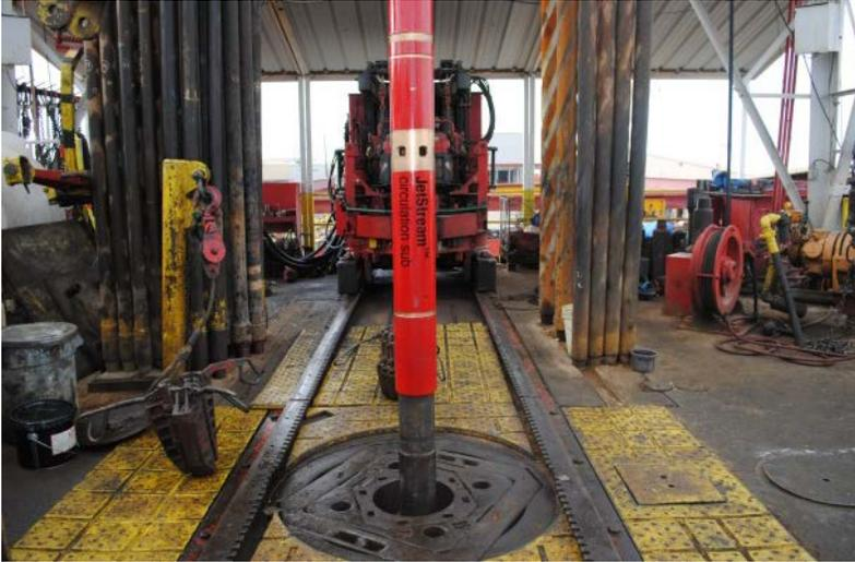
The JetStream RFID circulation sub, which enables selective, unlimited actuation that is not pressure-dependent, is well suited for drilling operations in porous and fractured formations.
