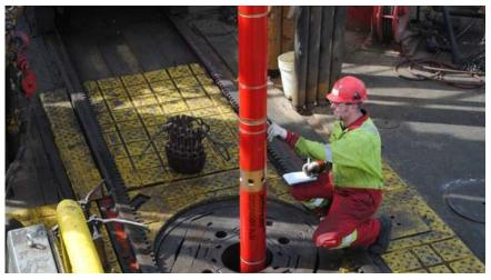
The JetStream RFID circulation sub has a large total flow area and no reduction in ID after actuation, which enables full through-bore flow and boosts annular velocity.
