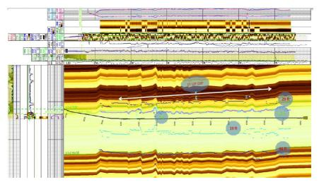
The image shows the well curtain section along the horizontal trajectory through the reservoir. The GuideWave tool enabled calculating the distance to bed boundaries, positioning the well trajectory close to the roof according to client requirements, and placing the well in the zone with the best pethrophysical properties.
