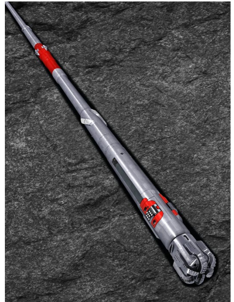
The Magnus RSS uses steering on and off to optimize the consumption and maintain trajectory.
