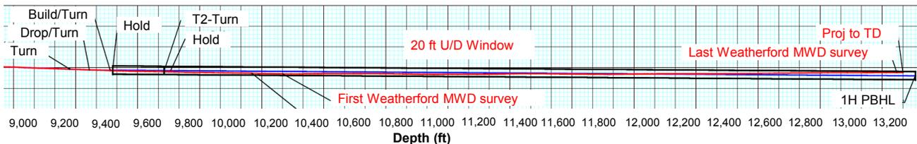
The Magnus RSS picked up where a conventional motor assembly left off and finished drilling the lateral section to the operator's desired depth.
