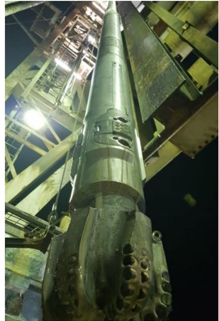
The Magnus RSS sidetracked off of a challenging cement plug in a single run.
