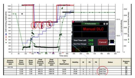
A good pressure point, it illustrates the seal with the formation and the drawdown/buildup showing repeatability and stability.
