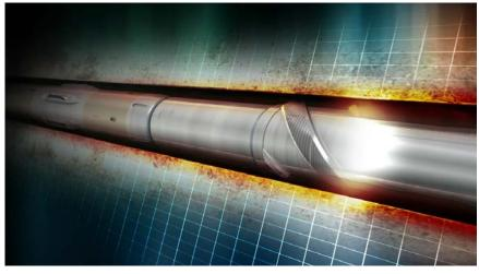
The Revolution Heat RSS executed a challenging well plan—including an 11°/100 ft (11°/30 m) dogleg—and set a client record for ROP while drilling in the Eagle Ford.
