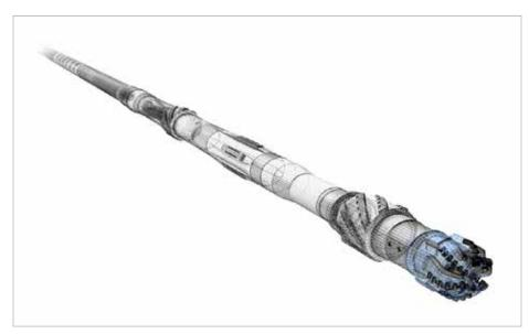
The Revolution rotary-steerable system (RSS) uses innovative point-the-bit technology to increase well value by providing superior wellbore quality and accurate wellbore placement while minimizing drilling risks. Unlike conventional push-the-bit systems, the RSS keeps the drill-bit face square to the rock and to the axis of the planned well path.
