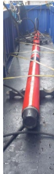
The loadout of the 7-in. JetStream circulating sub with a nozzled sub.
