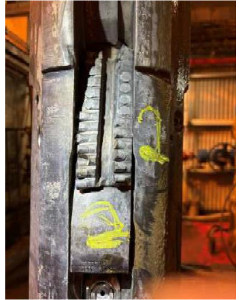
The 9 1/4-in. cutter blocks after the hole enlargement operation.
