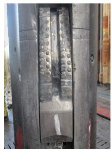
RipTide thermally stable PDC cutters provided superior strength and erosion resistance to deliver a full-gauge hole without failures. The, enlarged section enabled subsequent installation of liner and casing.
