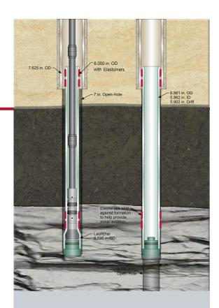
The Weatherford MetalSkin openhole liner system isolated a water-swellable shale zone located under existing 7 5/8-in. casing without cement, enabling the operator to drill to TD with minimal ID reduction and without increased NPT.
