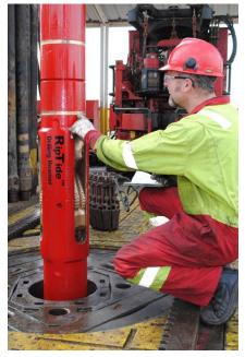
The Weatherford RipTide Rathole Killer drilling reamer can be activated by both pressure cycling and RFID to simultaneously drill and enlarge boreholes while eliminating ratholes.
