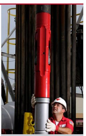
The innovative polycrystalline-diamond cutting structure and radio-frequency identification technology of the RipTide RFID drilling reamer maximize reaming efficiency and save rig time.
