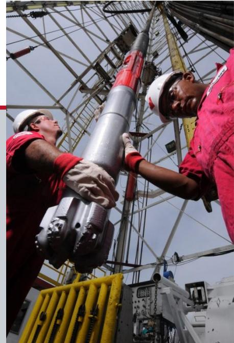
Weatherford's *RipTide* drilling reamer features RFID technology to enable on-demand activation and deactivation any time while drilling or tripping. The *RipTide* RFID model is the industry's first electronically controlled drilling reamer.
