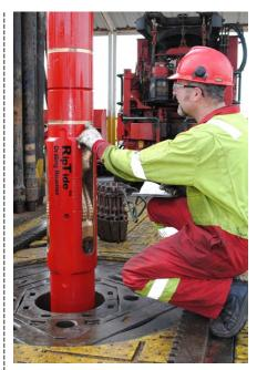
The RFID RipTide rathole killer drilling reamer can be activated by both pressure cycling and RFID to simultaneously drill and enlarge boreholes while eliminating ratholes.
