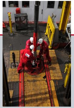
Weatherford used two *RipTide* RFID drilling reamers in tandem for independent, on-demand activation to successfully enlarge a 3,000 ft (914 m) section to the required 14 1/2-in. diameter and continuously drill a 12 1/4-in. pilot hole to total depth.
