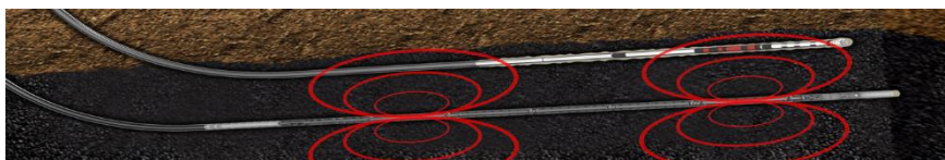
The Weatherford TwinWells ranging system accurately measures distances between drilling and offset wells
