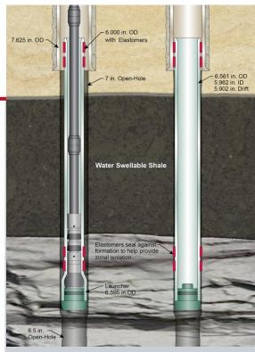
Weatherford's *MetalSkin* open-hole liner system isolated a water-swellable shale zone located under existing 7 5/8-in. casing without cement, enabling the operator to drill to TD with maximum hole size, seawater as a drilling fluid, and a stabilized wellbore.
